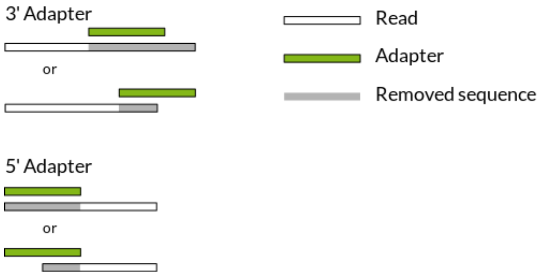
Figure 2: 3'- and 5'-adapter trimming ( source )
